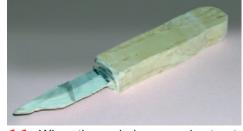
■ • When the resin has cured cut out and trim down the block to the guide lines, do not go over your guide lines.
