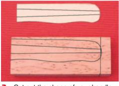
**3.** Cut out the shape of your handle and copy it onto the block by tracing around the shape, also repeating the marking of the tang
