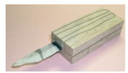
10. When you have achieved a good fit take apart ready for the bonding process. It is a good idea at the stage to polish up the bolster before mixing up a batch of epoxy resin (its much easier this way). Fill up the slot with as much resin as you can and reassemble, if you have a good fit excess resin will be extruded out of the slots and bolster joints, remove all excess resin with acetone (nail varnish remover) making sure that the bolster is very clean. Leave to cure as directed.
