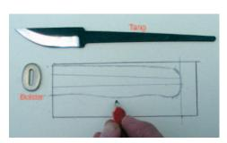
2. Using a thick piece of paper or light card, lay your block of wood down and trace around, marking off the amount of trim. The supplied bolster will determine the the depth of the handle closest to the blade. Plan you handle shape according to your needs and hand shape. Lay the knife tang down in the centre of your shape and draw round the edges.
