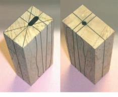
8. Now ream out the slot for the tang with a small rasp and pad or jap saw, joining up the from front to back, this is a gradual process, with repeated assembling for a good tight fit.
