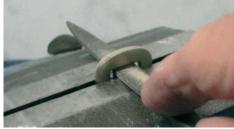
7. Clamp the bolster in a strong vice and carefully open up the slot with a it fits firmly.
