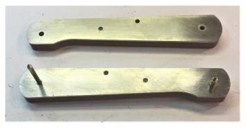
Separate the scales and lay down with the brass pin and one half of the pivot pin as shown.
