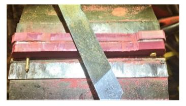
Join together and start filling down by hand, and then switch to a power sander to speed up the process, taking extra care not to damage or remove any metal.
