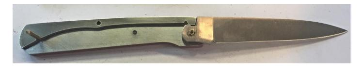
Apply another drop of oil to the heel of the blade **part 1**. Then position the other scale on top and squeeze together and tighten the pivot pin. The top of the spring **part 2** will now protrude, as shown below.
