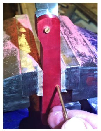
Make sure the pin is straight, and as soon as the point comes through, gently tap it, right through close to the scale. Take the knife out and test the action. Adjusting the pivot pin as desired.
