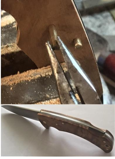
If you don't have access to a flatbed sander, use a piece of flat smooth metal and wrap your tungsten carbide paper around it for a good result. Remove the central pin before testing the mechanism. If the blade is loose, it will tighten when you peen the brass pins.
