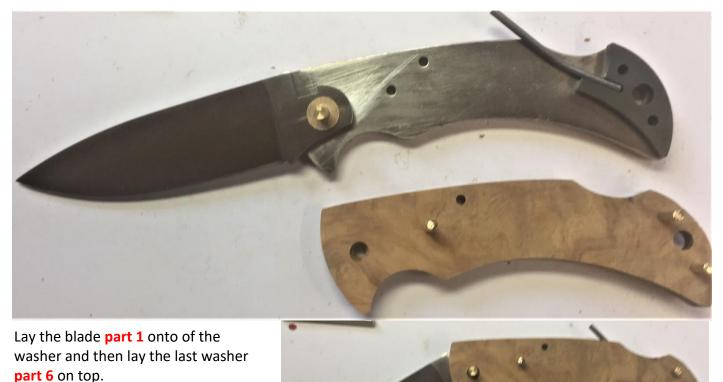
A small drop of thin oil on top of each wash will help the action later on. Now push on the scale locating the pins and squeeze together.
