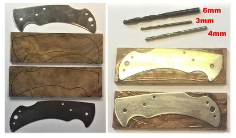
Lay the metal liners **parts 7 and 8** on your scales left and right and trace round the shape. Then using a good epoxy resin apply a thin layer of resin, to each surface and clamp to ensure a good bond. Remove any resin from the holes in the metal, with a cotton bud and nail varnish remover. This will make drilling easier. Allow plenty of time for the resin to cure.
