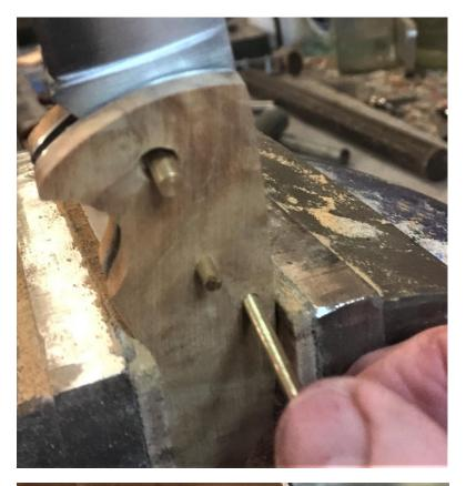
As soon as the holes are aligned push through the long tapered pin. A soft faced hammer will make it easy.
