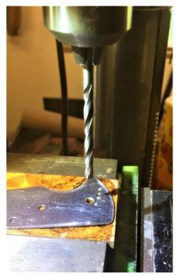
Its very important that the holes are drilled at right angles to your scales this will ensure that the kit will fit together properly. Drill the 4 and 3mm holes through from the metal side. Then turn them over and counter sink using a 6mm drill for the Pivot Pin and lanyard Tube parts **4**, **5 and 9**. Now cut out the shapes. And insert the brass pins as shown. The pins will hold the scales together while you file and sand them down.
