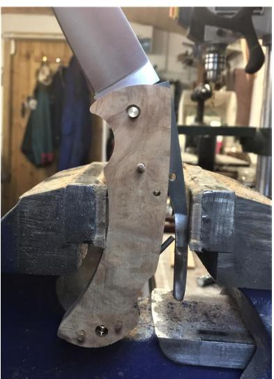
Insert the spring lever **part 2** into the heel if the blade **part 1**.
