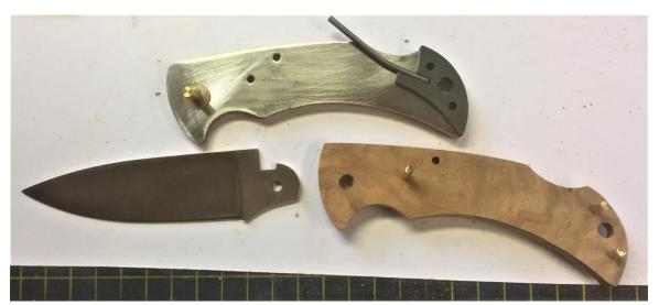
Insert the lanyard tube **part 9** at the same time. It helps to stabilise the other two brass pins.
