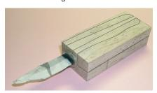
1 •• When you have achieved a good fit take apart ready for the bonding process. It is a good idea at the stage to polish up the bolster before mixing up a batch of epoxy resin (its much easier this way). Fill up the slot with as much resin as you can and reassemble, if you have a good fit excess resin will be extruded out of the slots and bolster joints, remove all excess resin with acetone (nail varnish remover) making sure that the bolster is very clean. Leave to cure as directed.
