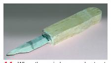
• When the resin has cured cut out and trim down the block to the guide lines, do not go over your guide lines.
