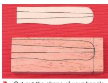
**3.** Cut out the shape of your handle and copy it onto the block by tracing around the shape, also repeating the marking of the tang
